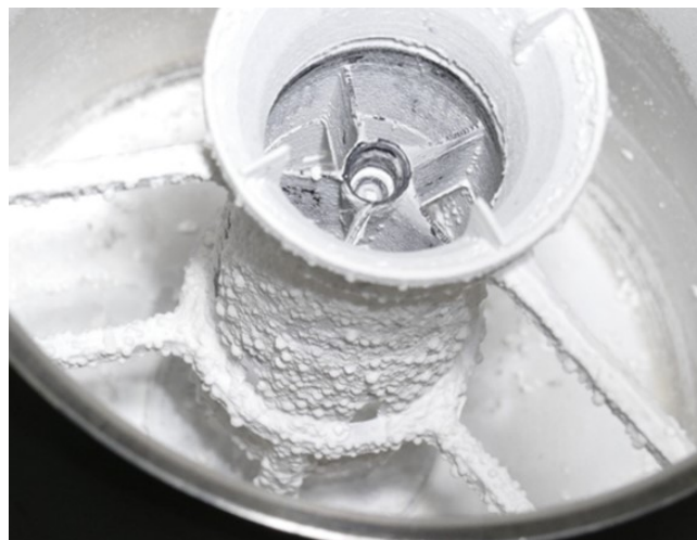
Figure 15. Visualization of scale formation on a laboratory draft tube tank.
